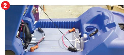
Compartment des batteries / Battery compartment
